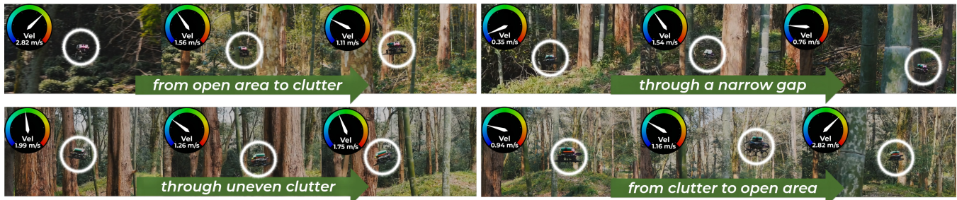
Fig. 1: Flight with agility adaptation in complex natural clutter. (Top left) The vehicle aggressively flies until it is near clutter, and further decelerates when observing a hidden bamboo behind a tree. (Top right) The vehicle flies cautiously when crossing a narrow gap between two tree trunks. (Bottom left) The vehicle flies smoothly between obstacles. (Bottom right) The vehicle flies aggressively after observing the open space in front of it.
